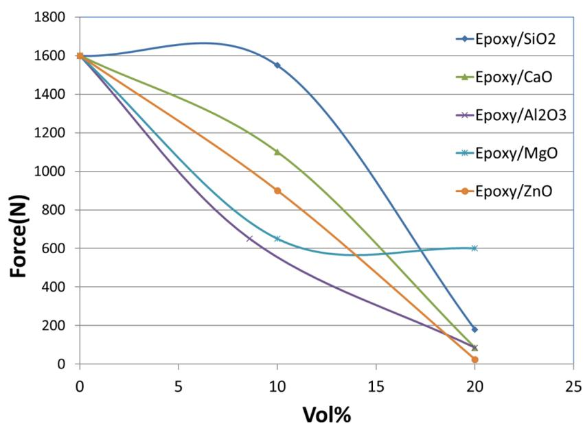
Fig.2. Lap-shear result
