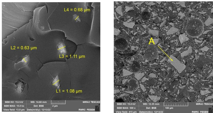
Epoxy containing 20 wt.%  $\text{SiO}_2$
